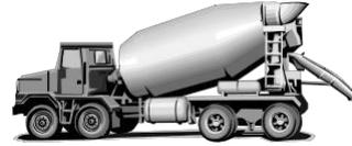
Ready Mix truck drivers are responsible for safely delivering concrete to the worksite and maintaining the quality of the concrete during transfer from plant to site. Trucks vary in size and design, and a fully loaded truck may weigh as much as 70,000 pounds and contain as much as 11 cubic yards of concrete.
